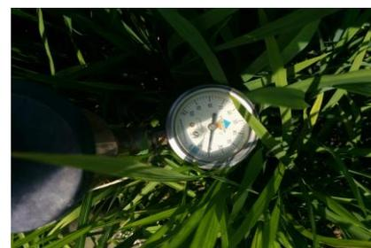
Figure 1 – Hydraulic tensiometer
