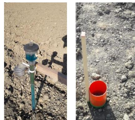
Figure 3 – Tensiometers and field water tubes installed in the Italian CS
