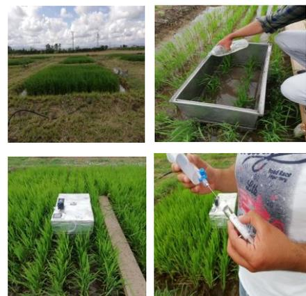
Figure 4 - Closed gas chamber used in the Turkish CS
